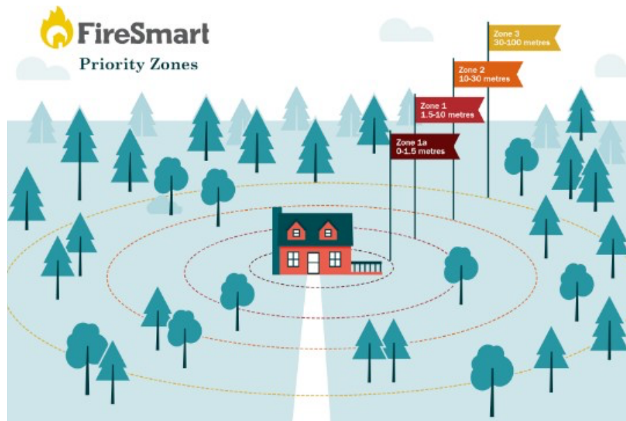
Figure 1 FireSmart Canada utilizes the concept of priority zones surrounding a home to help residents prioritize their hazard reduction efforts. A home's immediate surroundings (Zones 1 and 1a) are of immediate concern to the homeowner and should be targeted aggressively to reduce ignition hazards to the home.
